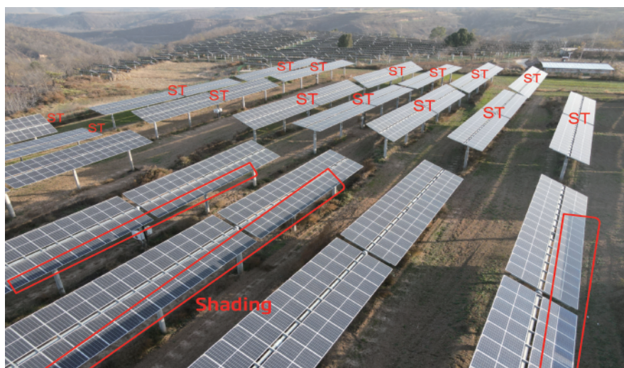
▲ Figure 11: Comparison of shading between using SuperTrack and the astronomical algorithm during the backtracking stage (The trackers marked ST in the picture are integrated with SuperTrack, while the trackers without marking are using the astronomical algorithm)
